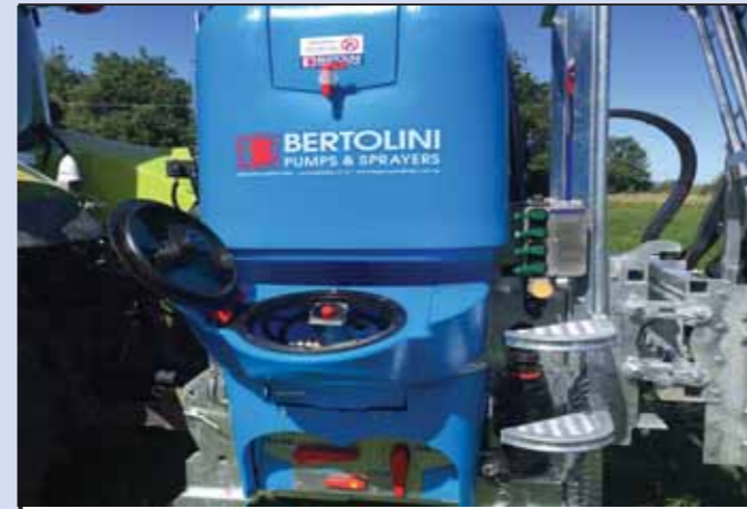
Rota-Mix 30, chemical induction hopper with container rinse function. Easy access controls at a safe working height.
