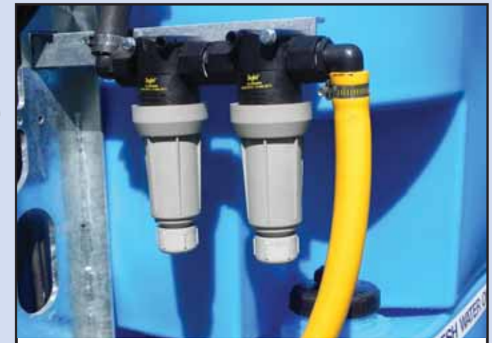
Dual sprayboom pressure filters, 80 and 100 mesh to eliminate individual nozzle strainers and blocked nozzles.
