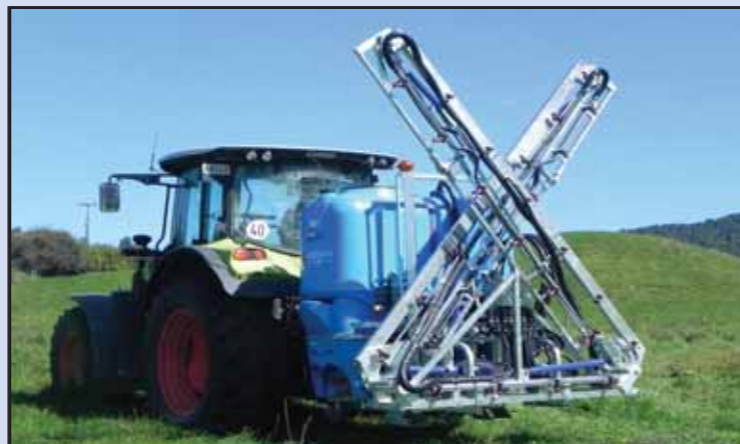
BA's new 12 or 15 metre "Super X-2" spray boom with wing tip lift and full independent hydraulic fold.
