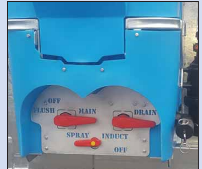
BA control station for spray/flush tank selection or chemical induction and tank drain.
