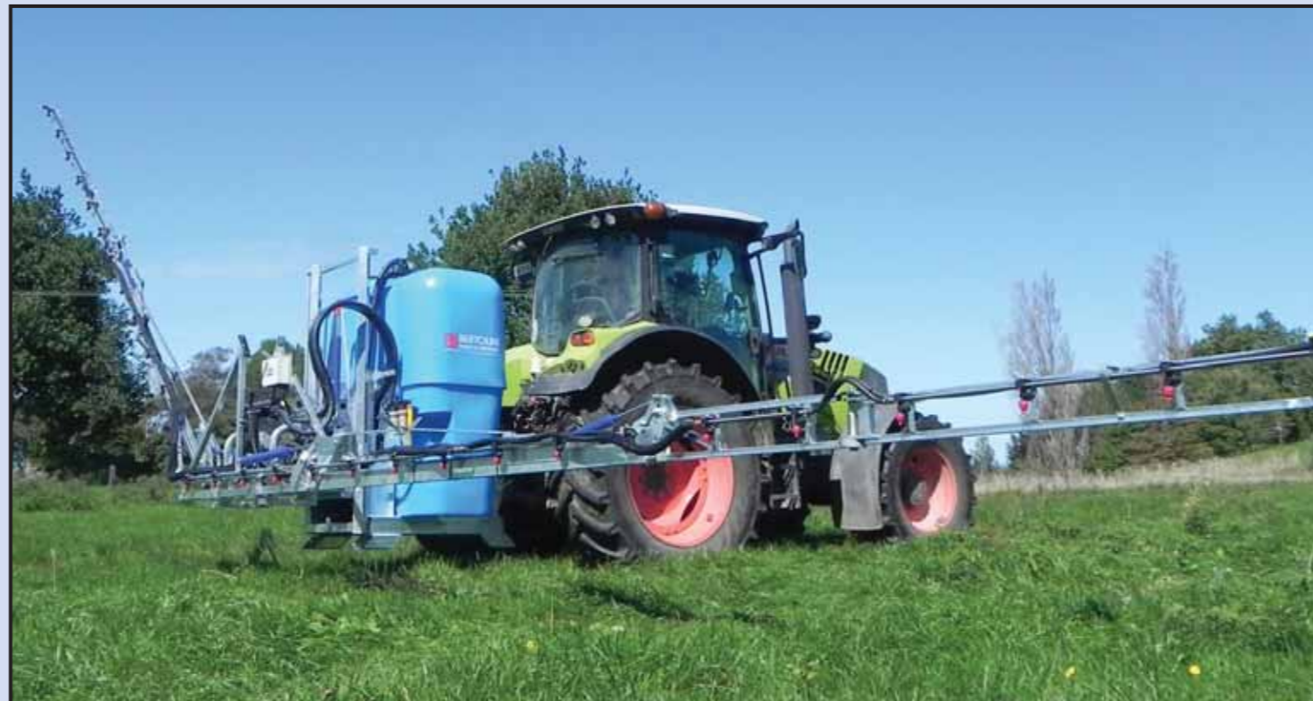
Rota-Mix 30, chemical induction hopper with container rinse function. Easy access controls at a safe working height.
