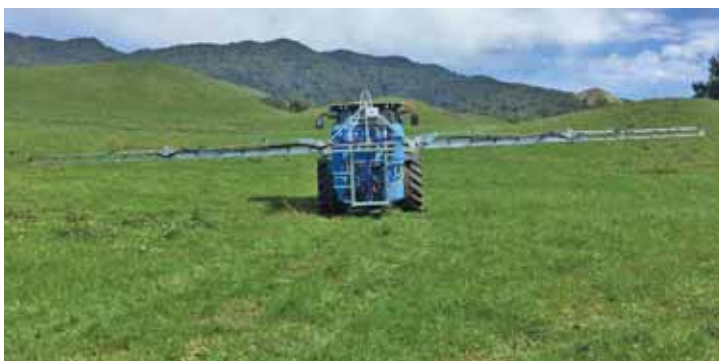
Optional hydraulic mast allows the operator to raise the boom 900mm.
