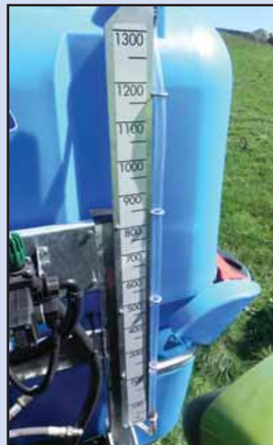
Bold tank level sight tube, easily read from the operator's position.
